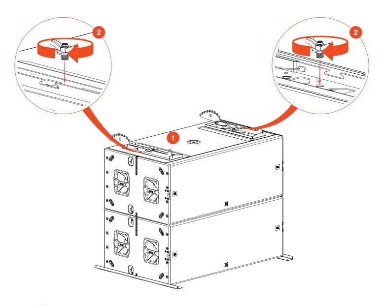
CAUTION: Safe limits for ground-stacked arrays always assume that the stacking surface (floor or stage) is flat. To avoid tipping hazards, do not deploy ground-stacked arrays on non-flat surfaces.
