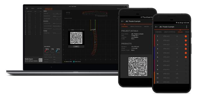
Once the system designer or lead tech computes the angles for each hang in LAC-3, every member of the crew can get the correct information for angles, attachment points, trim height, etc., either by scanning the QR code from LAC-3 directly with their device, or getting the data from a copy shared on another user's device. When all users onsite have the configuration data, arrays can be deployed quickly and efficiently.
