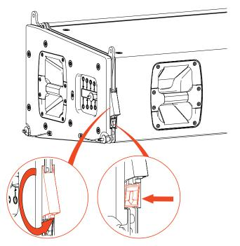
The system is locked when the red Locking lever is recessed into the cabinet. When the cabinets are suspended, a sequential locking sound is heard, indicating that the system has reached its final position and is locked. The system remains locked until the Angle Lock mechanism has been released.
