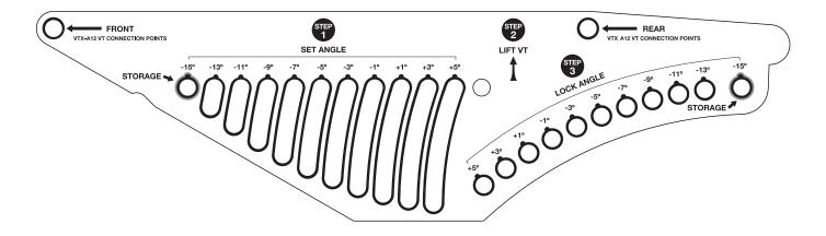
The Angle Selection mechanism settings correspond to the site angle of the VTX A12 enclosure connected to the GND (the bottom speaker of the array). For example, if -15° is selected on the GND, the bottom speaker of the array will point down at a 15-degree angle. If +5° is selected, the bottom speaker will point up at a 5-degree angle. These numbers are not related to the top enclosure of the array, and LAC-3 should be used to determine the overall angle of the ground stack.
