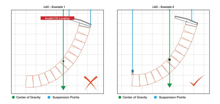
The two suspension points (motors) are used to adjust the array angle In this scenario, so the Array Frame's pick-point flexibility is not needed and a Suspension Bar can be used for the top frame, as well as on the bottom. This yields the same outcome with some weight and cost savings (LAC - Example 3).
