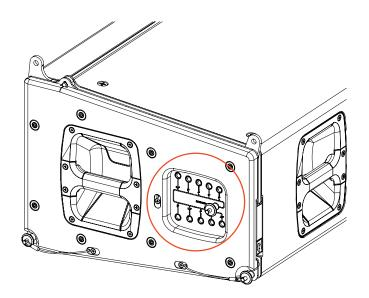
A dedicated quick release pin is used to select an angle. Angles are selected while the VTX A12 cabinets are on a VTX A12 VT resting on the ground. When the system is on the ground, the quick release pins are not under load and can be moved freely to a desired position.
