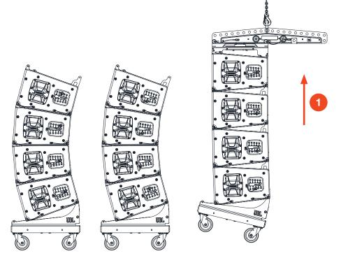
When all cabinet angles are set and the array is suspended a short distance off the ground, disconnect the Vertical Transporter (VT) by removing the two rear quick release pins, followed by the front pins. The array should not be so high in the air that the Vertical Transporter swings freely.
